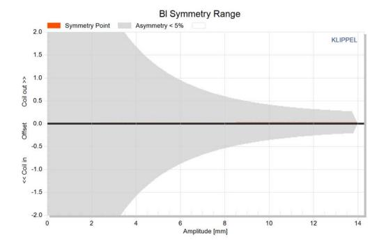
Figure 8: Bl Symmetry range measurement
