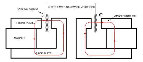
Figure 4: Traditional magnetic circuit with ISV coil
