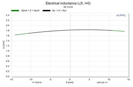
Figure 9: L(x) measurement of a Tetracoil speaker
