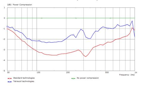
Figure 6: Power Compression Comparisons for single layer, ISV and Tetracoil technologies
