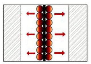
Figure 3: Interleaved Sandwich Voice-Coil
