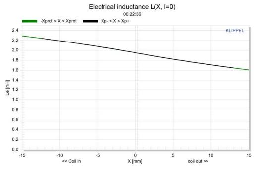
Figure 10: L(x) measurement of a traditional speaker
