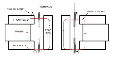
Figure 5: Tetracoil motor showing magnetic flux path flow
